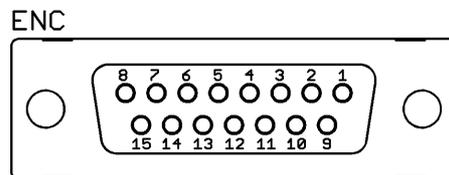
Figure 4: Encoder connector pin out (15 pin female D-Sub)
