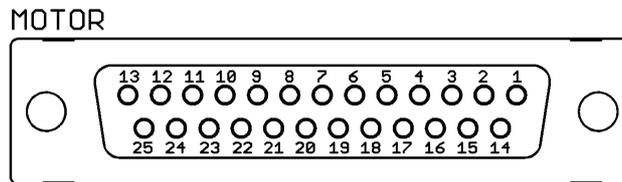
Figure 3: Motor connector pin out (25 pin female D-Sub)
