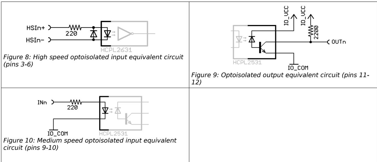
Note: In the schematics figures the shaded end represents drive logic side, which is insignificant from user's point of view.
