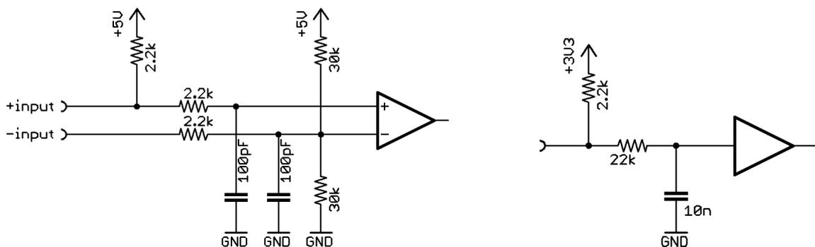
Figure 5: Equivalent circuit for differential inputs (pins 4-7 and Figure 6: Equivalent circuit for Hall sensor inputs (pins 1-3)
