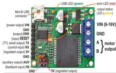
There are two different jrk motor controllers we have found that the Jrk 12v12 has an operating range from 6 V to 16 V. With a high continuous output current of 12 A (30 A peak) allowing us to control many medium-sized DC brushed motors with this board.
