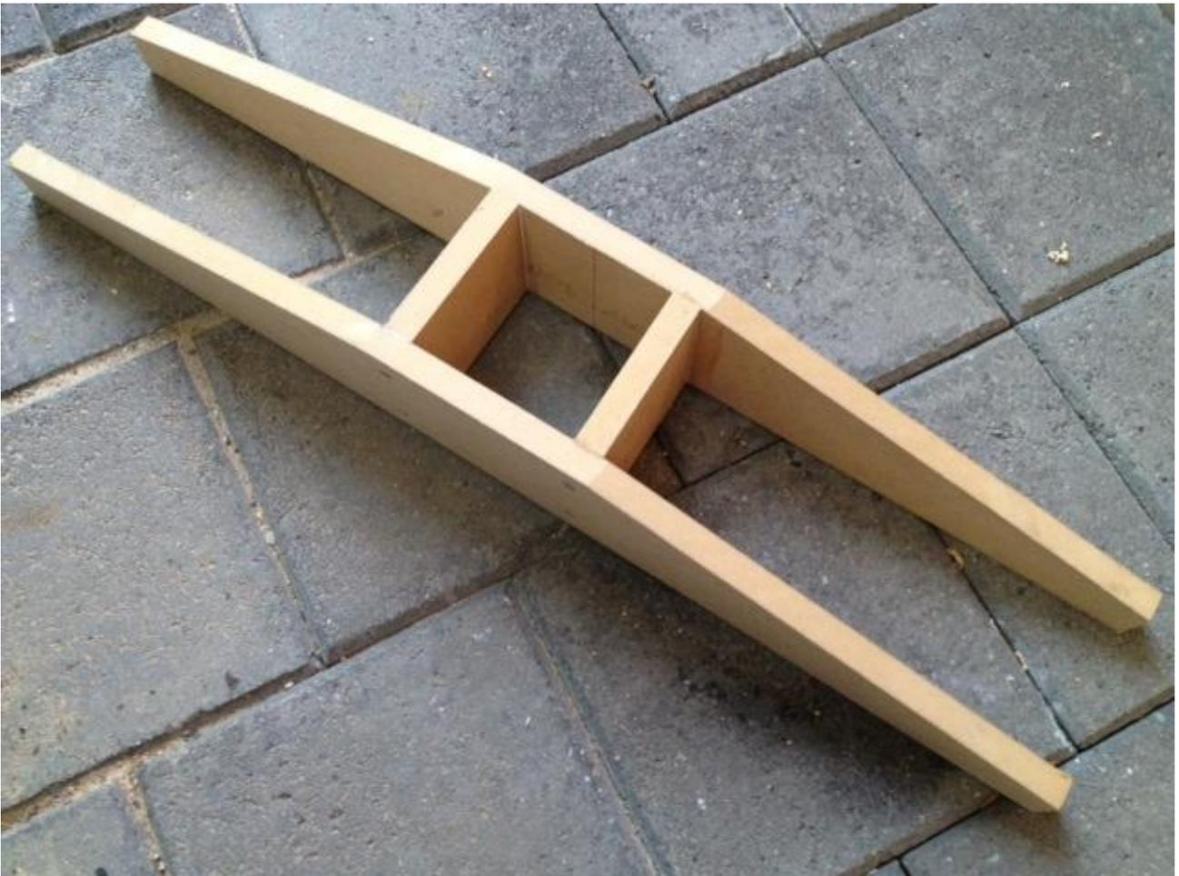
I cut the corners out before mounting the assembly into the base unit. This was to allow the cabling to run from the front to the back. Unfortunately I didn't make them big enough for the connectors and ferrites on the cable so I had a difficult job of trying to enlarge them later. I would now suggest cutting out a 20mmx20mm square out of the corners of the support assembly – but check the cables/connectors being used.
