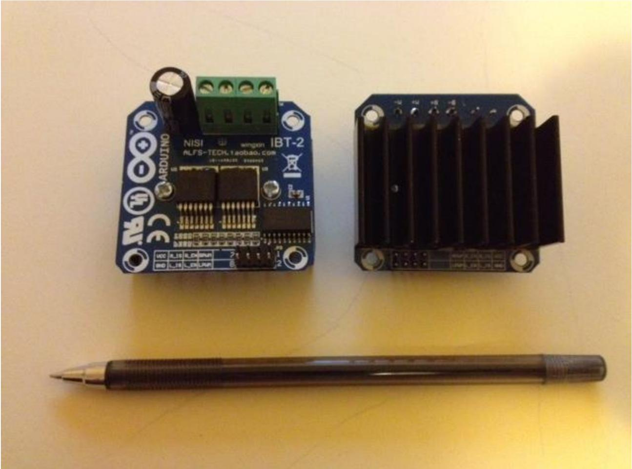
These H-Bridges have two sets of inputs for PWM, one for each direction. After a closer look at the circuit and BTS7960B datasheet I realized it was possible to use the inputs labeled R\_PWM and L\_PWM (which are actually the driver highside/lowside select inputs) for the motor direction inputs, and tie the R\_EN and L\_EN (the driver enable inputs) together and connect them to the Arduino PWM output. Refer to the wiring details.
