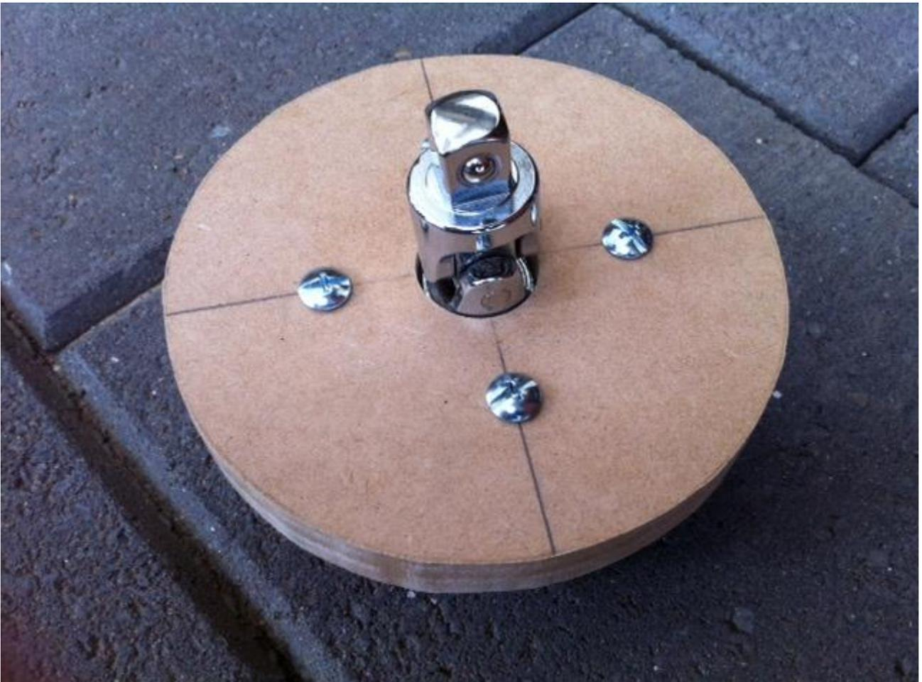
At this stage I made the seat platform square (600mmx600mm), later once everything was assembled I trimmed it down to taper the sides to the front of the seat. The photo below shows after I have trimmed it down. Be sure to mark the center of the platform as this is where the pivot mounts. The seat is later positioned on the platform to produce the best balance.
