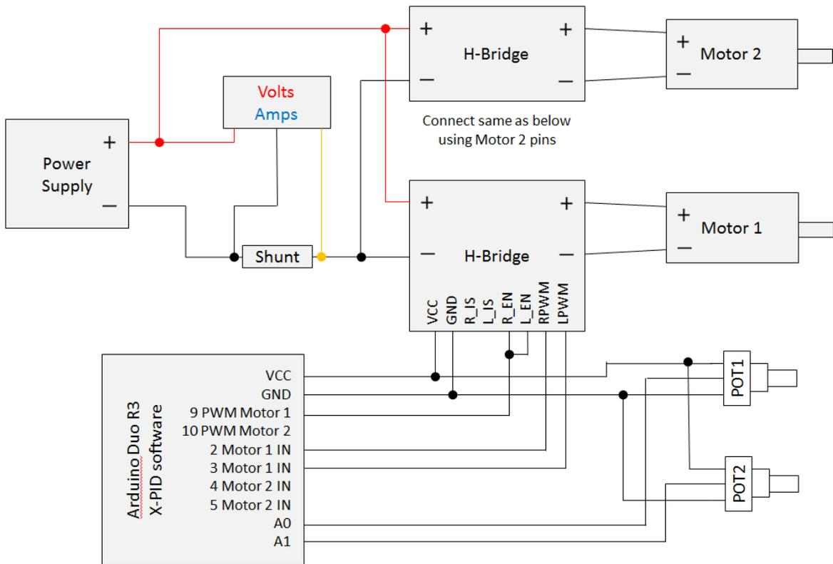
To make assembly and repairs/modifications as easy as possible I tried to use connectors as much as possible between the modules rather than solder directly to them. For the Arduino I used some prototype pcb to make a piggyback board that could be unplugged and all the wiring was connected to that. I have quite a stock of electronics at home so I didn't have to go and buy anything, but this does increase costs a bit.
