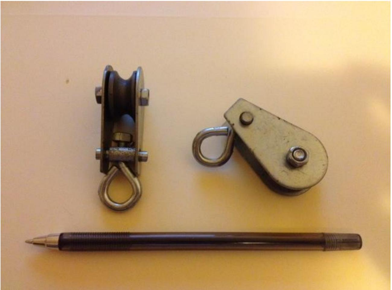
Next I modified 4 of the pulleys so that they could be mounted in a vertical position bolted directly to the base of the simulator. To do this I pulled the pulleys apart and bent the metal side plates outward and then reassembled them. See below:
