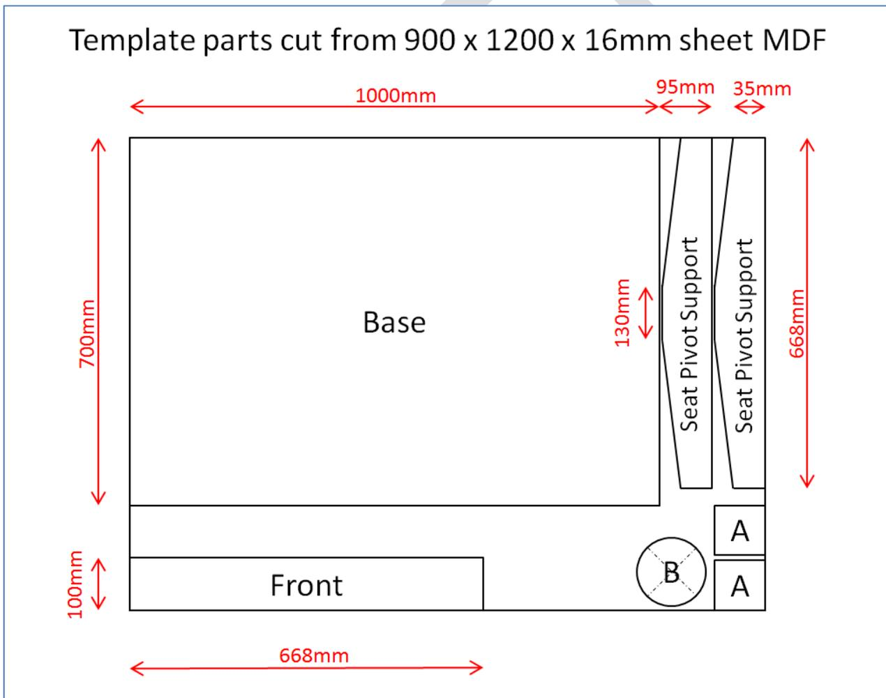
Template parts cut from 600 x 1200 x 16mm sheet MDF
