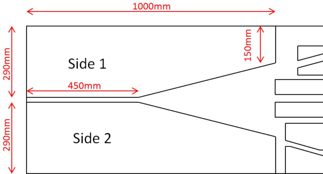
Template parts cut from 600 x 1200 x 16mm sheet MDF
