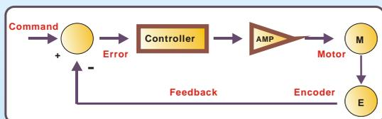
Most step-motor-based motion systems operate in open loop providing position control without feedback. When step motors move loads in open loop a potential loss of synchronism between commanded steps and actual steps may occur.
