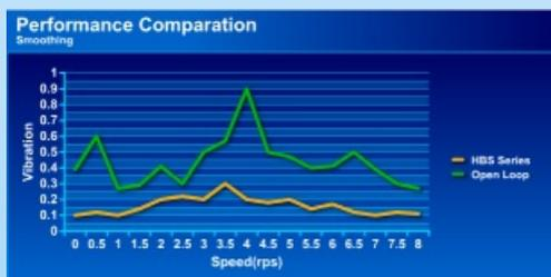
Unlike a conventional Micro step drive, the on-board high performance DSP (Digital Signal Processor) performs vector control and filtering, producing a smooth rotational control with minimum ripples.
