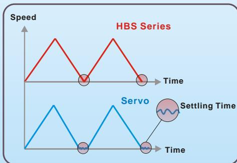
HBS series instantly synchronizes with command pulses providing fast positional response. HBS series is the optimum choice when zero-speed stability and rapid motions within a short distance are required. Traditional servo motor systems have a natural delay between the commanding input signals and the resultant motion because of the constant monitoring of the current position, necessitating in a waiting time until it settles, called settling time.
