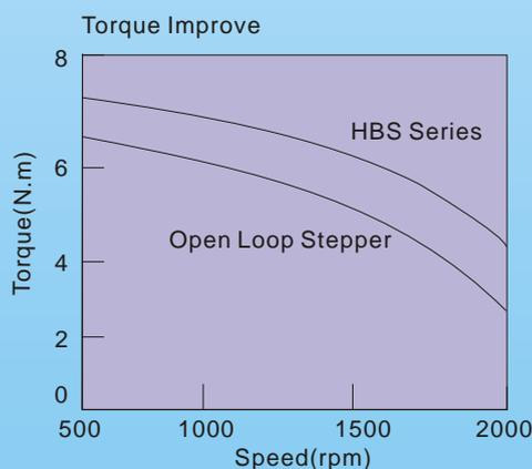
Torque improvement increases torque up to 30% at high speed, therefore they can drive a normal stepper motor to 3000 RPM or even higher, and significantly increase production efficiency.
