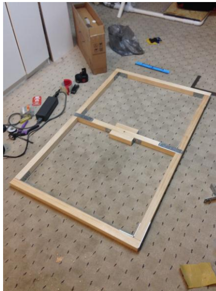
Seat-Frame with center beam to attach to rubber pivot
