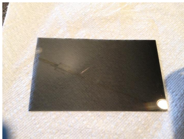
Privacy screen-filter cut down to 7" diagonally to fit the Oculus Rift's display
