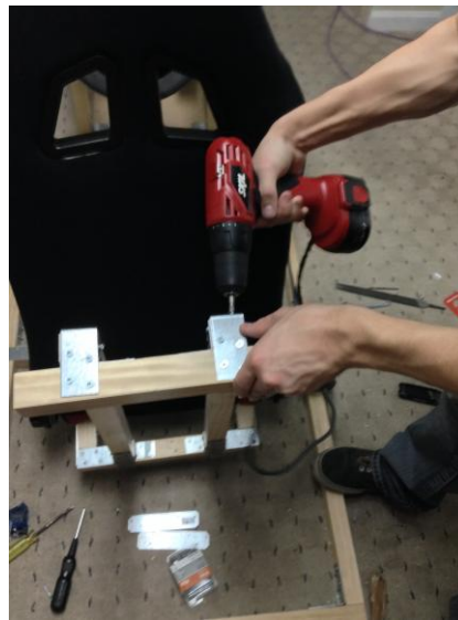
Mounting actuators and actuator mounts to seat-frame
